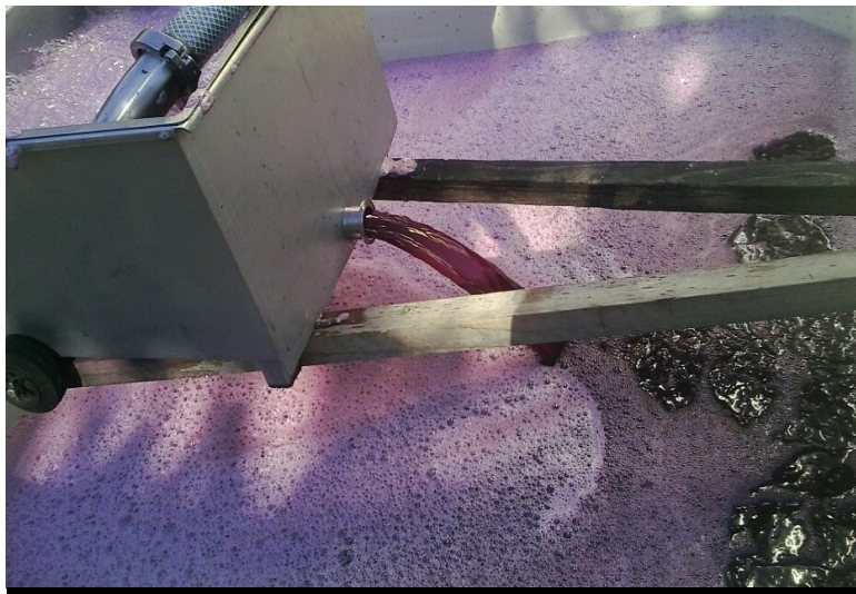
To circulate fermenting juice of red wines from the bottom of the tank over the skin cap that forms during fermentation to ensure optimal extraction and prevent bacterial spoilage.
